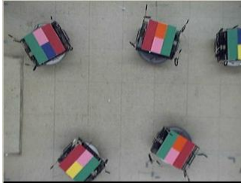
Figure 4.7: The webcam shot of the testbed. The color patch on each node uniquely identifies the node as well as tells its position and orientation.
