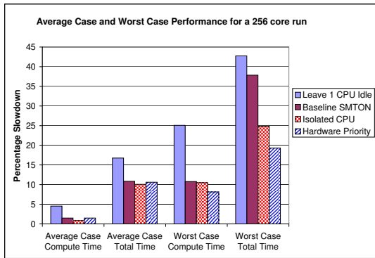
Figure 8. Average case and worst case performance of the parallel benchmark for the 256 core run
