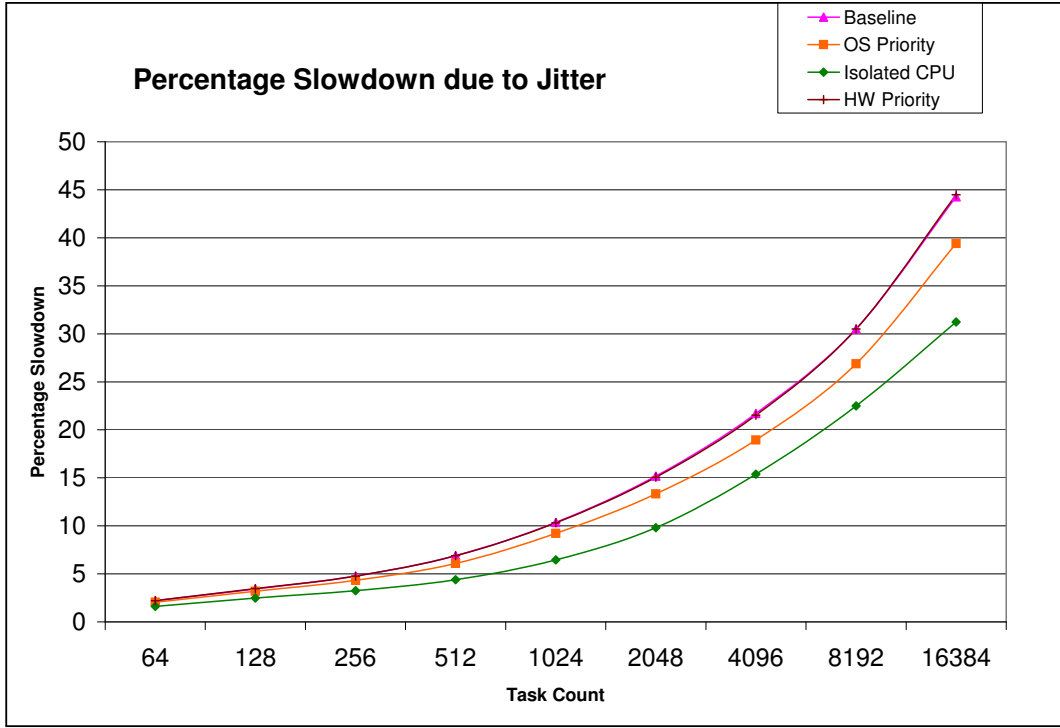
Figure 4. Simulated percentage slowdown due to jitter
